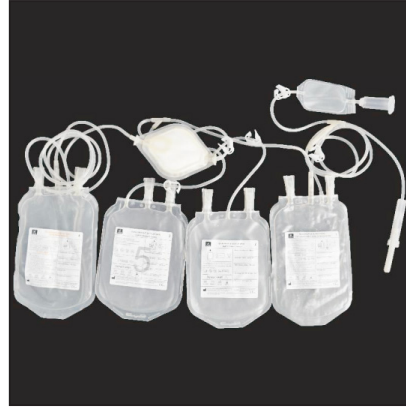
Quadruple blood bags with CPD+SAGM, with RBC leukocyte-reduced filter, PDS and NPD (calendered film)
